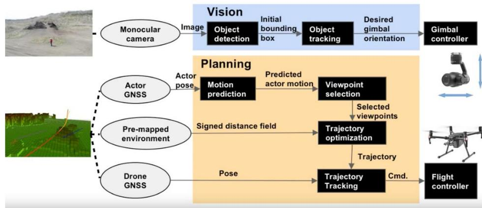
**Figure 98: Example of an AI drone video filming system<sup>513</sup>.**
