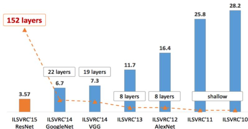
**Figure 54: Evolution of CNN architectures<sup>212</sup>. The object recognition rate (%) of each network is depicted as a bar.**
