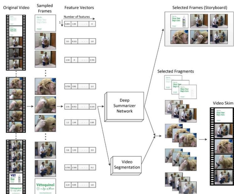
**Figure 63: High-level representation of the analysis pipeline of deep-learning-based video summarisation methods for generating a video storyboard and a video skim.<sup>260</sup>**
