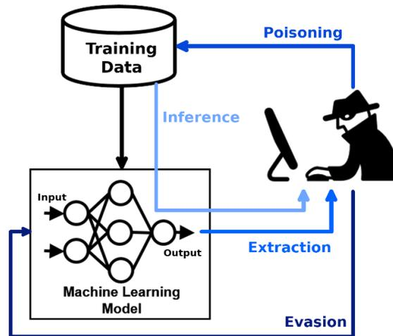
**Figure 75: Different types of attacks against machine learning models.**<sup>327</sup>
